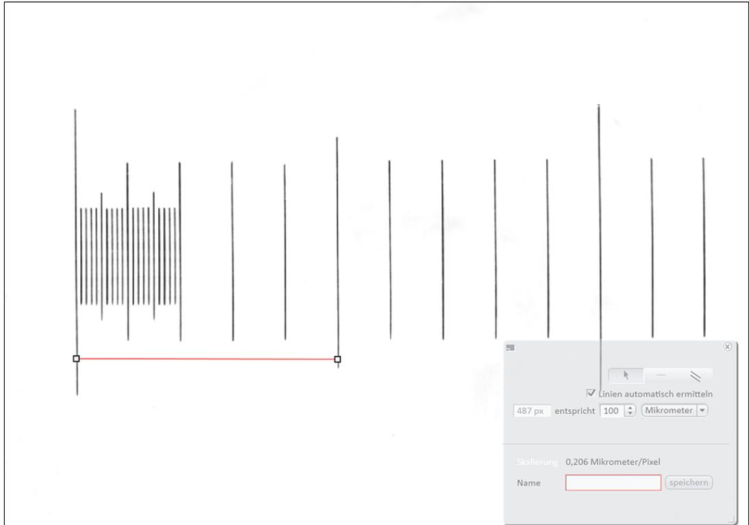
6. Enter the true distance between both scale lines in the calibration wizard. In our example this is 500 micrometer.
