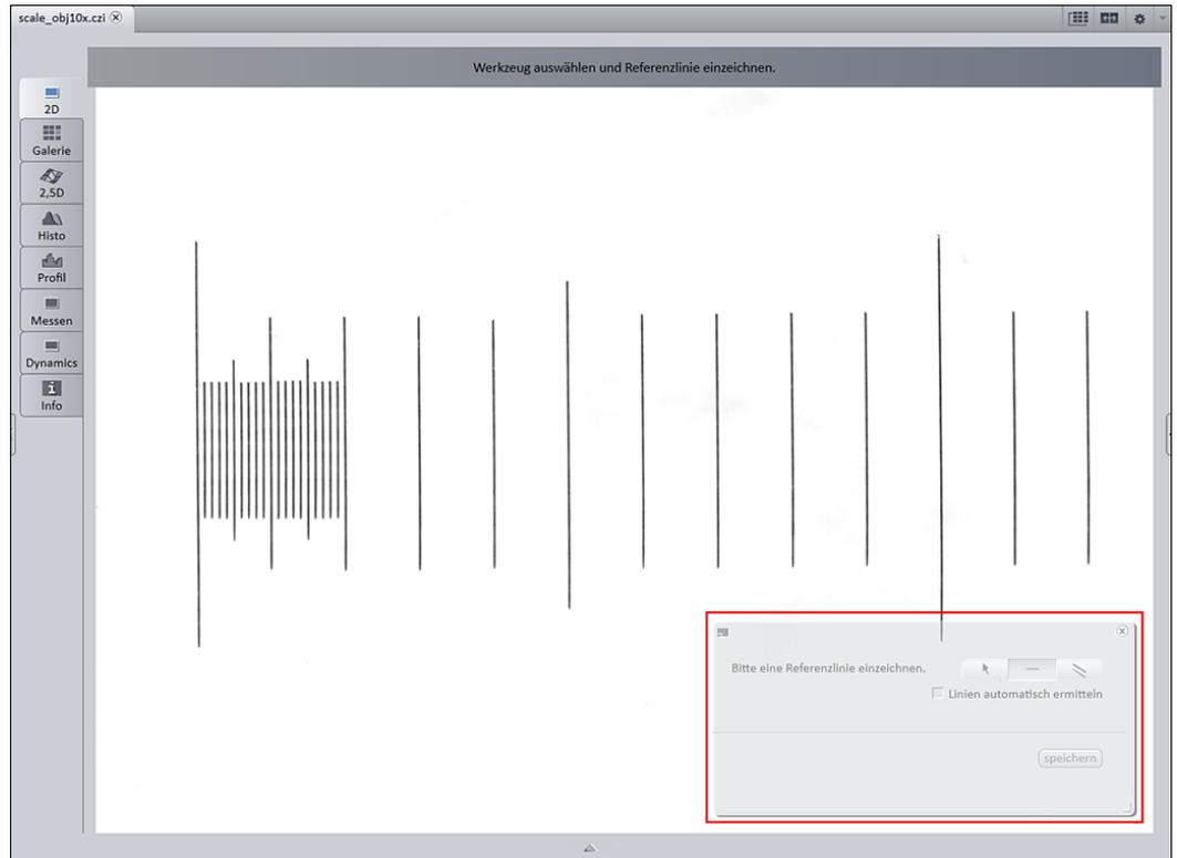
4. Click on **single line** button as reference line in the calibration wizard and activate the **automatic Line Detection** button.
