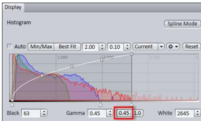
2. Move the controls under the display curve left and right in order to directly adjust the values for **Brightness (White)**, **Gamma**, and **Contrast (Black)** in the live image.
